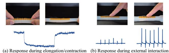
Fig. 1. Wrinkle-based soft sensing system with tactile perception: (a) Embedded strain gauge's orientation, as well as electrical response change resulted by self-deformation. (b) The sensing system can sense adaptively various states of interaction, such as indentation or sliding, by changing the morphology of wrinkle.
