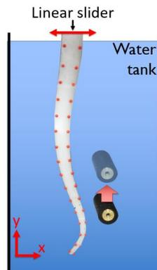
Figure 1. EcoFlex 10 octopus inspired, passive silicone arm submerged in water. The proximal end was attached to a linear slider with a sinusoidal input signal that excited the arm without touching the object. The object was moved to different locations. Simple linear regression was sufficient to learn to classify different positions of the object by simply observing the bending of the arm (proprioceptive sensing).
