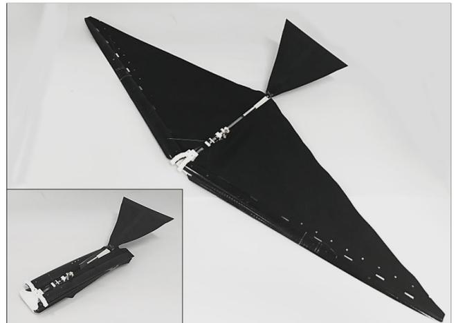
Figure 3. Deployable glider module for multimodal robots
