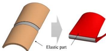
Figure 1. Bio-inspired curved compliant facet origami structure
