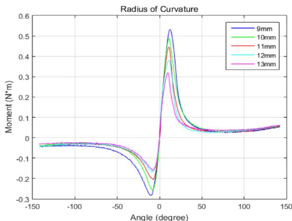
Figure 2. Experimental result of the folding angle v.s. joint torque of the curved compliant facet origami structure
