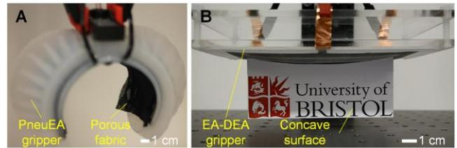
Figure. (A): prototype of a PneuEA gripper, grasping a flexible and porous fabric from a convex surface; (B): prototype of a self-sensing EA-DEA gripper, grasping a concave surface.
