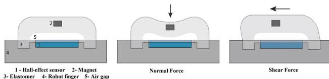
Fig. 1. Sensor design scheme
