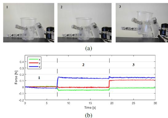
Fig. 2. a) Lifting a plastic cup in three phases. b) Sensor response in time.
