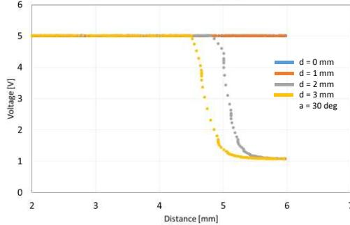
Figure 9. Characteristic curve of output voltage of optical fiber in case of  $a = 30^\circ$  and changing  $d$
