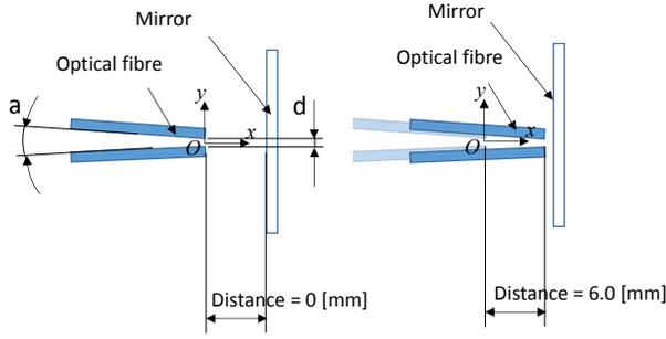
Figure 5. Experiment setup of the optical fibres
