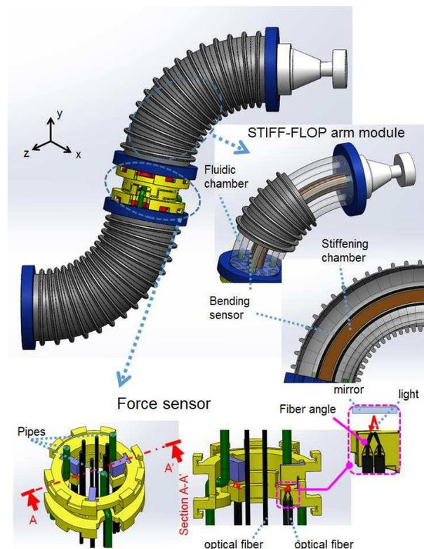
Figure 1. Overview of the STIFF-FLOP manipulator and three axis sensor
