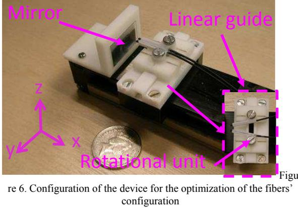
Figure 6. Configuration of the device for the optimization of the fibers' configuration
