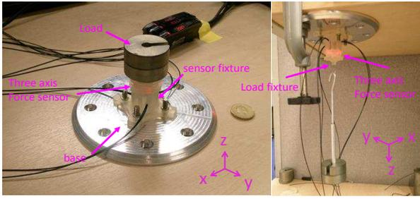
Figure 10. Experimental set-up for the calibration of  $F_z$ .
