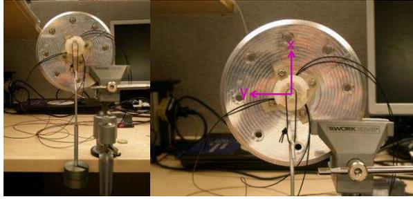
Figure 12. Experimental set-up for the calibration of  $M_y$ .
