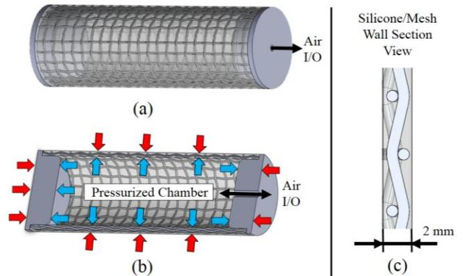
**Figure 1:** CAD drawings of the stiffness-controllable link: overview of the link assembly (a), longitudinal section view of the link (b) showing the I/O channel for pressurized air, with azure arrows showing the force distribution of the pressurized air inside the internal chamber and red arrows the force distribution of the reaction forces of the link. (c) subfigure shows a longitudinal magnified section of the wall link, showing the mesh embedded in a 2 mm silicone layer.
