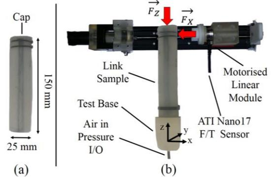
**Figure 3:** Link sample with 3D printed cap embedded for stiffness test (a) and setup for the lateral stiffness tests at the tip (b): direction of the lateral force  $F_x$  and of the longitudinal force  $F_z$  applied during the tests are marked.
