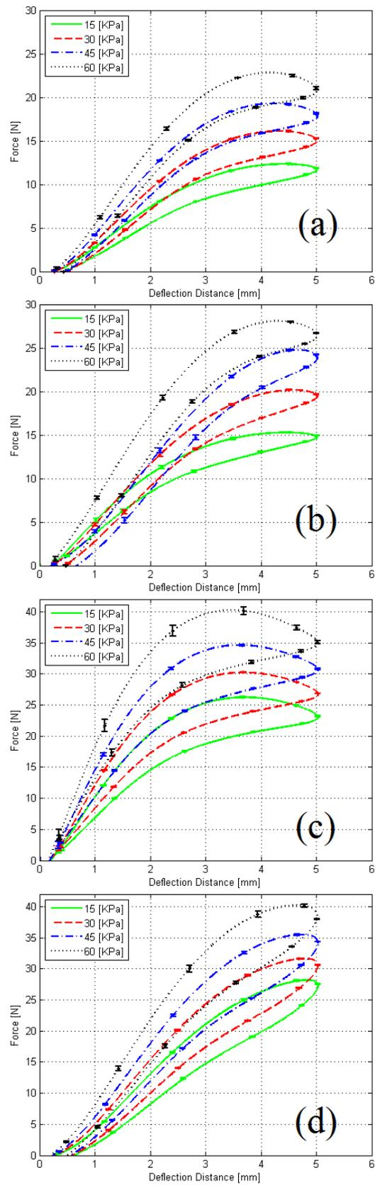
**Figure 5:** Deflection versus force at the link tip longitudinally applied for samples (a), (b), (c) and (d) at 15KPa, 30KPa, 45KPa and 60KPa.
