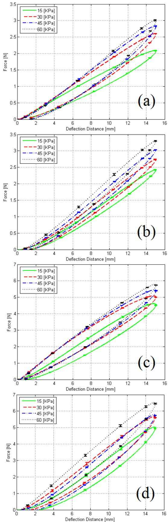
**Figure 4:** Deflection distance versus force at the link tip laterally applied for samples (a), (b), (c) and (d) at 15 KPa, 30 KPa, 45 KPa and 60 KPa.
