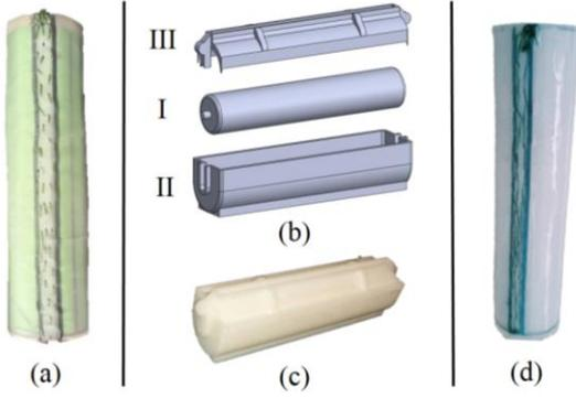
**Figure 2:** Fabrication stages of the link: mesh sewn in the shape of a cylinder (a), mould components (I, II and III (b)) and mould assembled (c). Figure (d) shows the link after demoulding and removing of the silicone excess.
