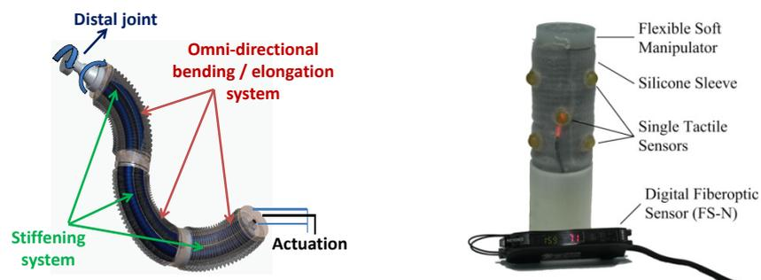
**Figure:** CAD drawing of the overall architecture of the STIFF-FLOP manipulator (left) and one single soft manipulator module of the stretchable sensor sleeve with multiple tactile sensors (right).
