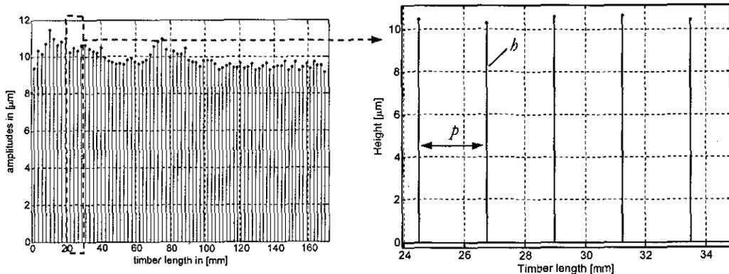
Fig. 5 Re-created surface profile by using spindle speed
