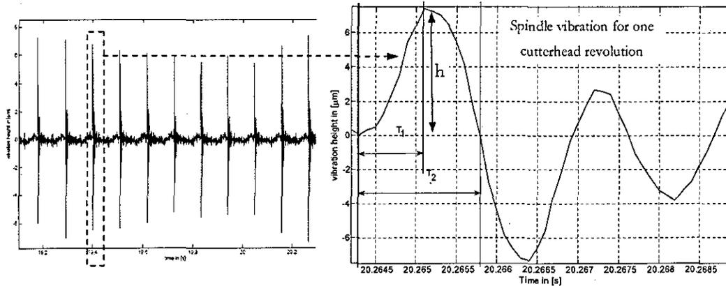
Fig 6: Spindle vibrations during the machining process
