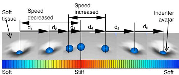
**Fig. 1** Pseudo-haptic feedback: modification of the cursor speed when passing over a hard nodule ( $d_1 > d_2 > d_3$ ,  $d_3 < d_4$ ).
