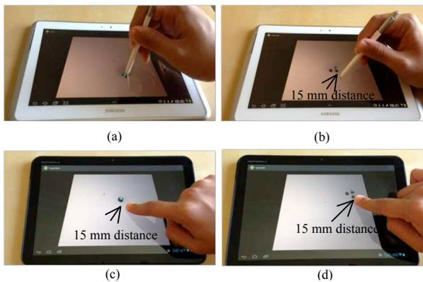
**Fig. 3** Pseudo-haptic palpation: (a) single-fingered palpation using a tablet and an S-pen; (b) multi-fingered palpation using a tablet and an S-pen; (c) single-fingered palpation using a tablet and a bare finger of the user; (d) multi-fingered palpation using a tablet and a bare finger of the user.
