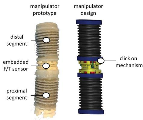
Fig. 1. STIFF-FLOP two segments manipulator with its own modular structure and the embedded 3 d.o.f. F/T sensor.
