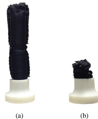
Fig. 1. Prototype of the new bio-inspired, antagonistically actuated and stiffness controllable manipulator in the (a) stiff and elongated and (b) entirely shrunk state.
