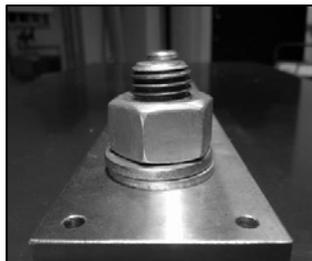
Fig. 12. The ‘two washers’ error scenario. The 2<sup>nd</sup> washer will cause an error detection within *stage 3* or *4*, since the desired angular position of the nut will not be reached.
