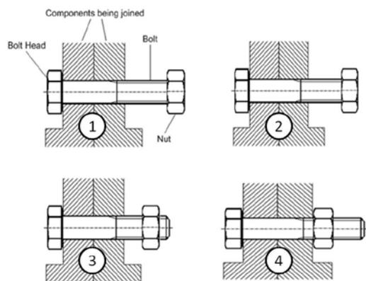
Fig. 2. The 4 stages of the bolt tightening process [17, 18].
