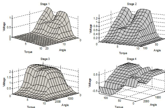
Fig. 10. From the top left to the bottom right panel, the  $s$  Stage 1, 2, 3 and 4 membership functions with their linguistic rules, respectively.
